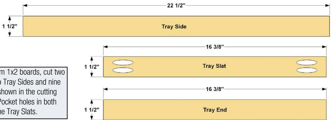
**Step 15:** From 1x2 boards, cut two Tray Ends, Two Tray Sides and nine Tray Slats, as shown in the cutting diagram. Drill Pocket holes in both ends in all of the Tray Slats.
