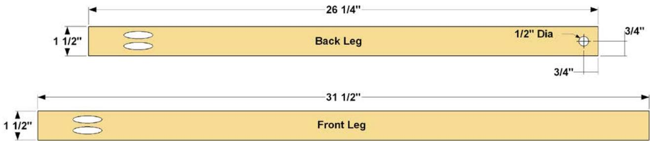
**Step 4:** Cut two Front Legs and two Back Legs to length from 2x2 boards, as shown in the cutting diagram. Set your pocket hole jig for 1 1/2" thick material and drill a single set of pocket holes on one end of the Front and Back Legs as shown.
