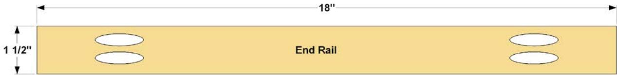
**Step 8:** Cut seven End Rails to length from 2x2 pine boards as shown in the cutting diagram. Set your pocket hole jig for 1 1/2" material, and then drill pocket holes in both ends of each Rail.
